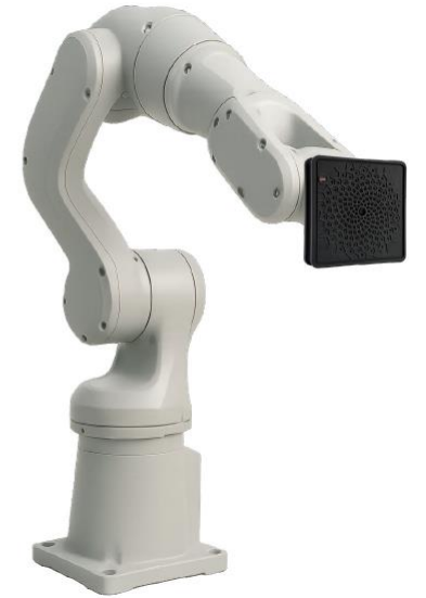
6-axis industrial robot arm with the SoundCam Ultra 3 sensor
