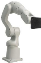
6-axis industrial robot arm with the SoundCam Ultra 3 sensor
